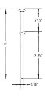
17" Heavily plated hanger of 3/16" wire, shaped to stay securely on a rod, and to take maximum abuse.
