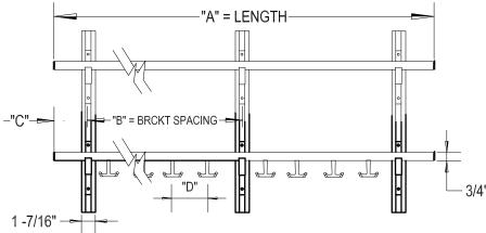
WALLSTRIP SECURMENT HOLES: DRILL TO FIT A #10 ROUND HEAD SCREW (WALL FASTENERS BY OTHERS)
